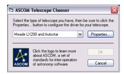
Choose your telescope model from the list, press the **Properties** button, and select the serial port that your telescope is connected to
